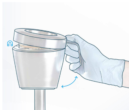
Figure 1: Aseptic operation during air sampling using the magnetic perforated lid with handle, keeping hands out of the critical zone.
