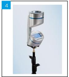
In case you are using the MAS-100 Eco for air sampling: Attach your air sampler directly to the tripod with the tripod adapter.
