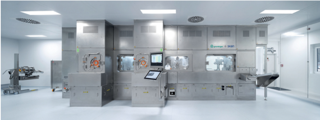
Figure 4: Gloveless isolator “robocell” with integrated Rapid-C + (source: SKAN and MBV).
