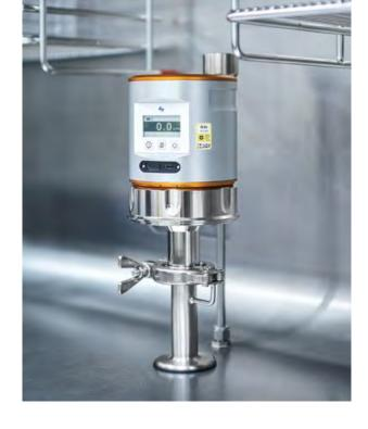
In any case, we ensure that the calibration of your air sampler can be traced back to international standards via the certified MAS-100 Regulus digital anemometer and via our ISO 17025 accredited calibration laboratory.
